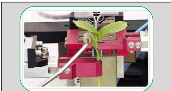
Matching part Matching correctly against rootstock and scion
