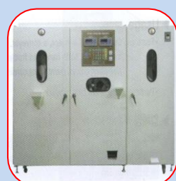
Protein Analyzer and Paddy automatic examiner Measuring protein content and rice quality
